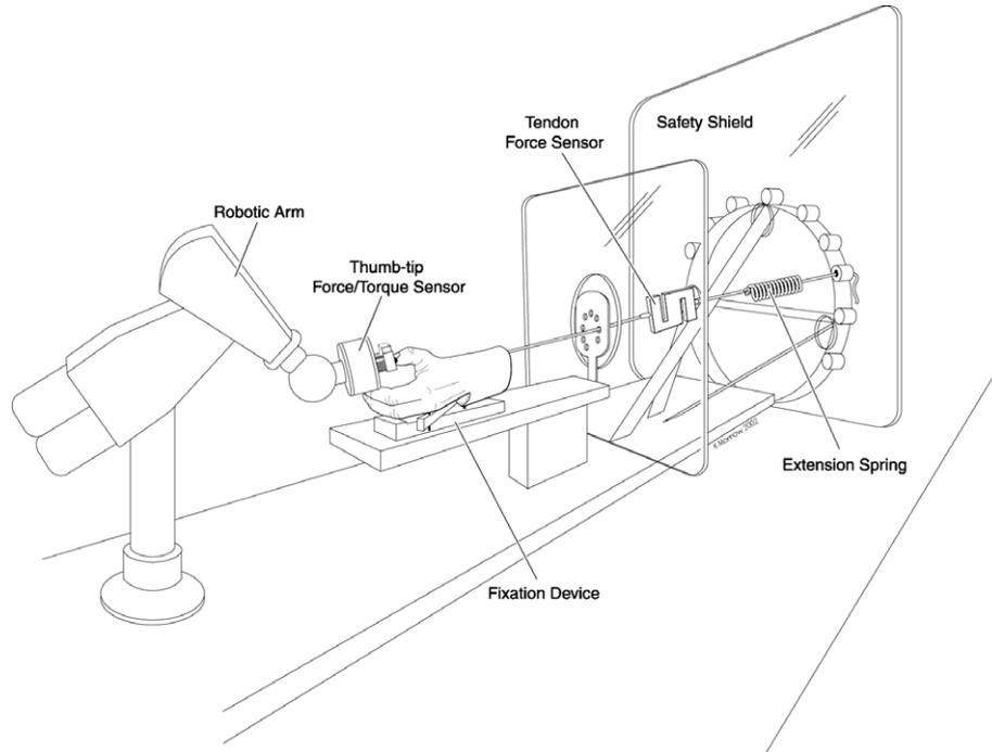
Fig. 1. Experimental setup. The distal upper extremity of each specimen was mounted on a frame to a fixation device, and the thumb to the end of a robotic arm. Force was applied to the muscle’s insertion by stretching the attached extension spring. The in-series tendon force sensor measured the applied force. The resulting thumb-tip force was measured by the six-axis force/torque sensor rigidly attached to the thumb-tip.
