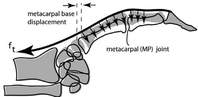
Fig. 2. Effect of tendon force on thumb posture. The pull of the tendon pushes the MP joint into less flexion as base of the metacarpal moves into the wrist due to the mobility of the carpal bones. A flexor tendon would produce a similar result through the action of tendon pulleys.
