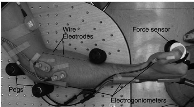
**Figure 1.** Top view of the experimental setup. The subject's arm is resting at shoulder height on the shelf with adjustable pegs that limit elbow position (showing the externally supported condition). The location of the Br is marked on the subject's forearm and the electrode insertion sites are identified. The force sensor is mounted to a custom grip the subject is holding. Electrogoniometers record the position of the elbow, wrist, and metacarpophalangeal joint of the thumb.
